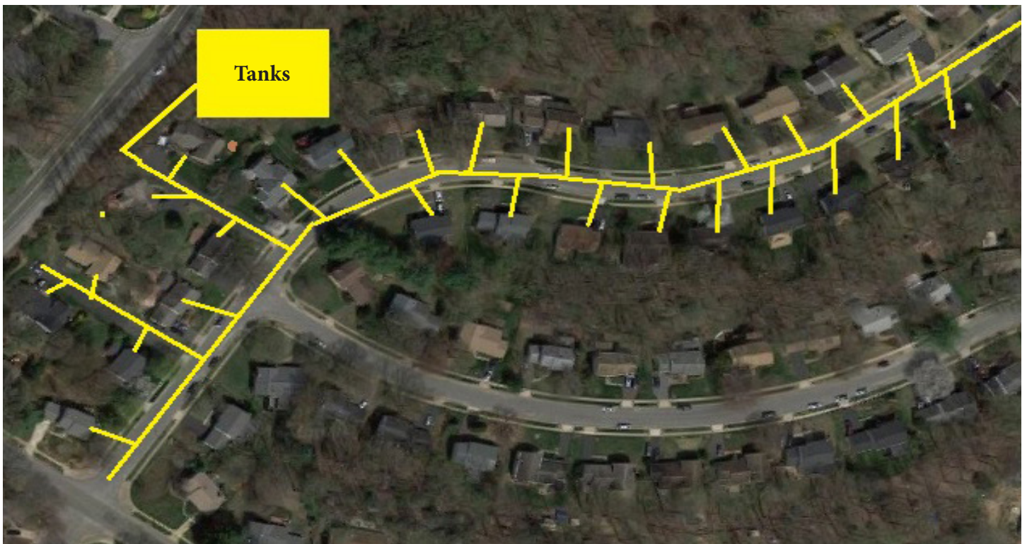
Figure 1 - In this example of Scenario A, a section of the neighborhood pictured above is served by an LPG system. The yellow box near the top of the picture represents the operator's tanks, which are connected to the homes by mains and service lines represented by the yellow lines.
